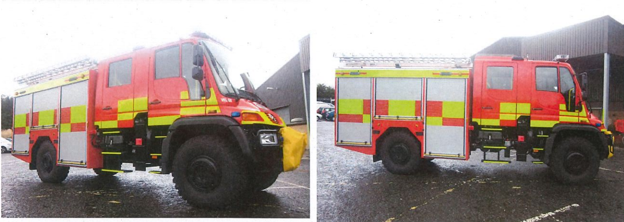
Examples of Unimog vehicles adapted from military and forestry specifications into fire appliances, in a range of sizes, suitable for off-road travel.
