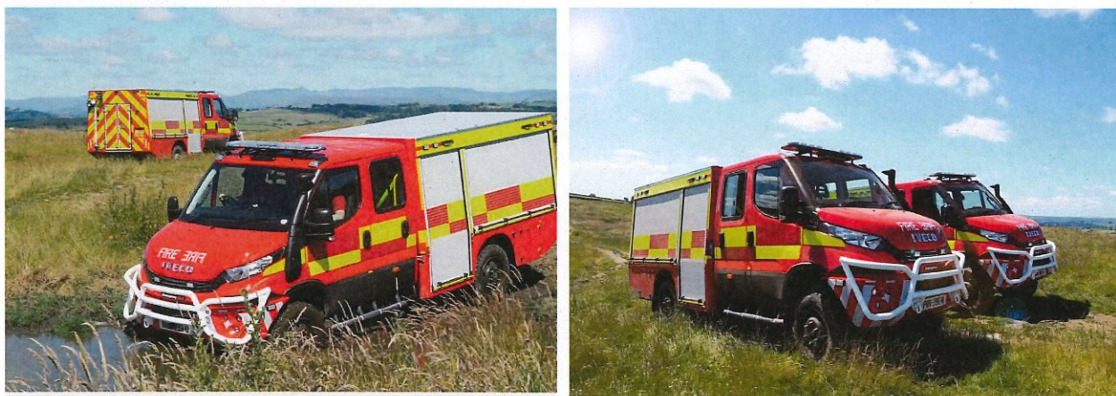
Examples of a 7.5 tonne fire appliance which offers similar capabilities to a standard fire engine but with better access to hard-to-reach areas due to its reduced size and all-wheel-drive capabilities.
